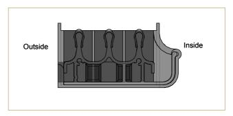
The bottom rail profile must be placed center of the structure on ground.
