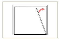
There is no hole on top and vertical profile. Before of the fixing you should make a hole on "first layer" on top and vertical profile. Then you can fix by M5,5x50mm self-drilling screw for each meter.
