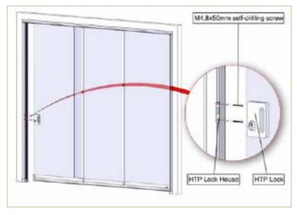
5.8. HSM Lock System Installed to glass panel
