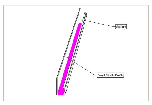
After the applied a sealant to panel middle profile now you can place to glass panel as you see at below. The brushes should be assembled to each other correctly.
