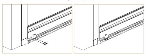
Pin must be inserted properly.
