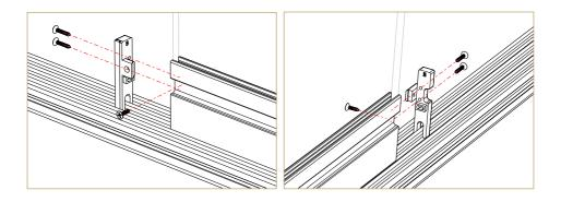
Place a sliding end cap to end of panel joint profile then fix by related screws.
