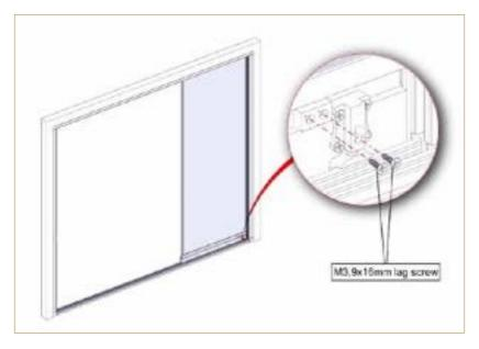
5.6. First Glass Panel Lock System Types Inner Lock System M3,9x16mm lag screw
