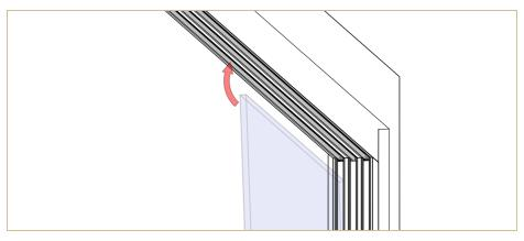
Then, lift up the glass panel and place the wheels to the bottom rail.
