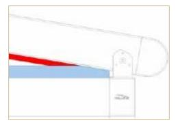
After cutting process you must fix F Profile to bottom of the rail by M4,8x25mm self-drilling screw.
