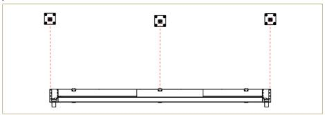
After connection of the wall flange, hanging pie must connect to the wall flange.
