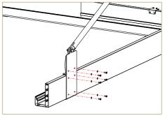
Also, you should fix from inside with bended bracket by nut.
