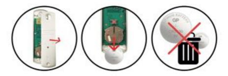
Using a small screwdriver loosen the screws on the reverse side of the remote control and remove the back cover.
